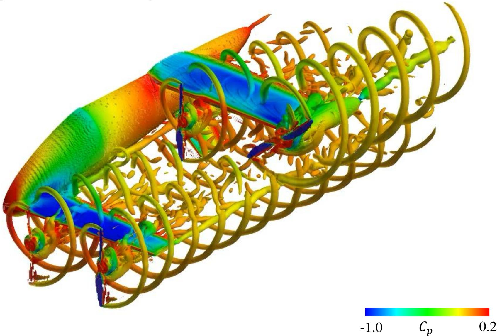
We conducted URANS for the wingtip-mounted propeller and eVTOL with DEP to clarify the propeller effect and validate prediction accuracy.
