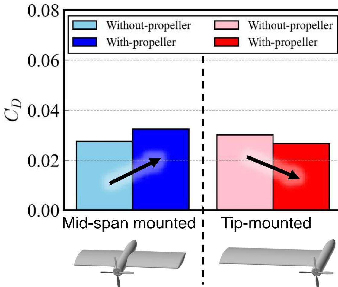
**Mid-span mounted propeller increases  $C_D$  of wing and nacelle, while tip-mounted propeller decreases that.**
